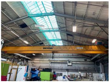
Champion Street 5ton single girder overhead crane, 10m approx span, pendant control (1995)
