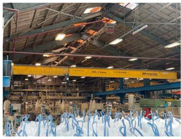
Demag 1ton single girder crane, 3.5m approx span, pendant control (2005)
