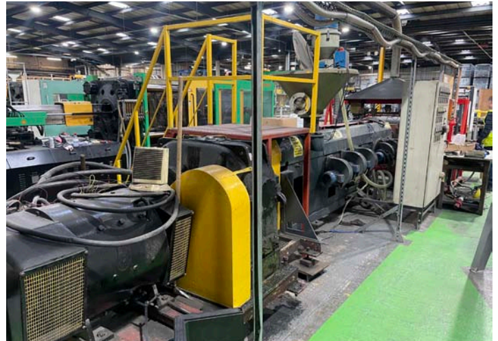
Boxer extrusion line inc: extruder, hopper, top & bottom heated rollers, accumulator, slit / rewind station etc [019]
