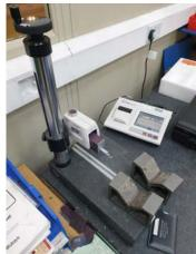
Mitutoyo SJ-410 surface roughness tester with digital control & printer 2x Olympus Delta BX41M-LED laboratory microscope.
